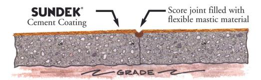
During the early 1990s, SUNDEK invented a system that takes advantage of the natural movement that occurs along these lines rather than trying to "Mess with Mother Nature." These scorelines are placed directly over the cracks in the deck allowing them to move naturally. They are sealed with a flexible material to prevent moisture from penetrating the deck. SUNDEK professionals then complete the pattern with decorative scorelines in the uncracked portion of the deck.
