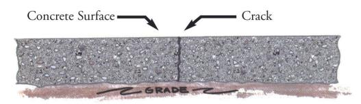
A structural crack occurs where stress has developed in a concrete deck. These cracks then begin to move as the concrete heats and cools (expands and contracts). Trying to end this motion is expensive and ultimately unsatisfactory.
