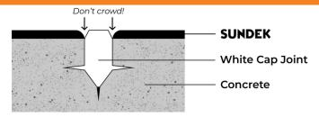
SUNDEK is feathered down to the edge of the white cap or 1/2 inch plastic place joint allowing some relief at the edge. The PVC white cap is left exposed, no mastic needed. May be finish coated.
