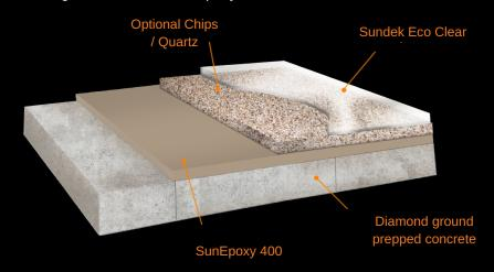
**Surface Preparation:** If cracks are present, fill with CrackRepair 100TM (see CrackRepair 100TM Tech Data Sheet for detailed instruction). Mechanically grind or chemically etch the surface to CSP 2 to 3 profile. Please note that for porous floors, an additional prime coat may be necessary to ensure proper adhesion of chips as well as the coating.
